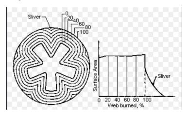
This example shows how the burnlines will move throughout the rocket, however our motor has a different starting shape.
