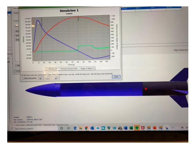
The nose cone is 30", with a base diameter of 13" and a wall thickness of .25". The nose cone is a Haack Series Van Karman Ogive shape for maximum efficiency, which was derived using the openrocket simulator, and can be printed via solidworks by being generated on Matlab. The matlab generation code is . Unlike the body, the nose cone is made out of steel in order to move the center of gravity of the rocket above the center of pressure.
