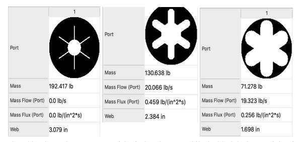
The white shows the empty area of the fuel or the port, while the black is the remaining fuel left to be burnt. The inner circle within the port has a starting radius of 1.6" and eventually grows to accommodate the entire cylinder.
